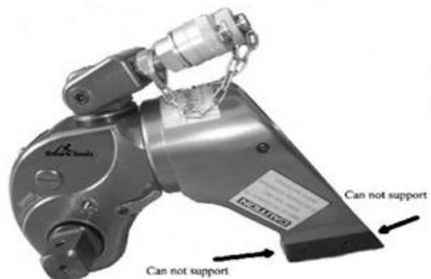
from the swivel inlets. It will always be toward the lower half of the housing and on one side of the housing when tightening and the other side when loosening.
